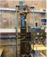
Technology for P recovery as struvite starting from pig manure digestate with fluidized bed crystallization system (ID:256)
